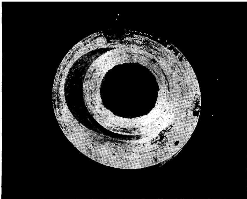
FIGURE 24.—Muzzle bushing. (Can be made quickly of wood and faced with tin or sheet iron for extra strength.)
