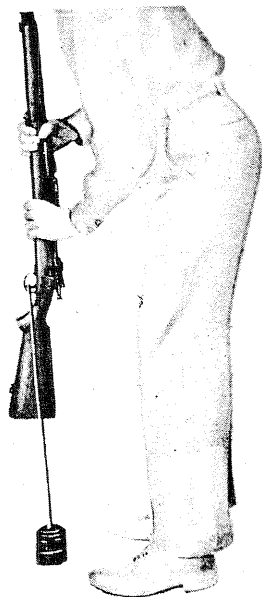
Figure 62 — Testing Trigger Pull
