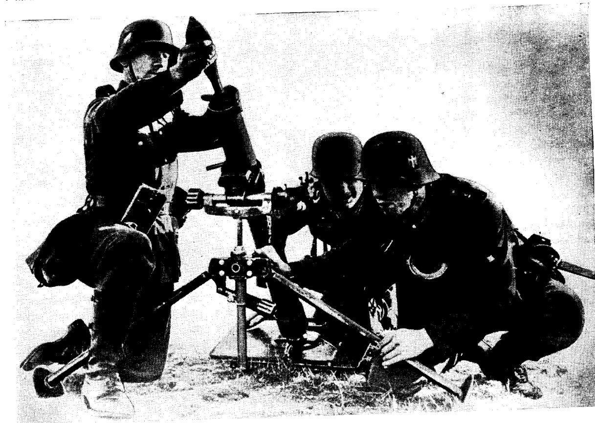
Figure 23.—8 cm schwerer Granatenwerfer (81-mm mortar) in action.
