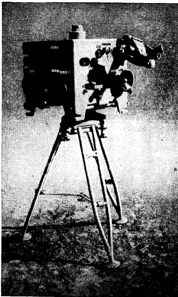
Figure 69.—Kommandohilfegerät 35 (anti-aircraft gun director) used as an auxiliary.
