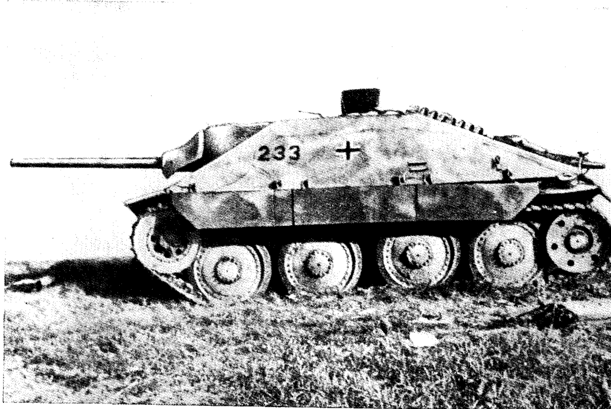
Figure 81.—7.5 cm Pak 39 (L/48) on Pz. Jäg 38.
