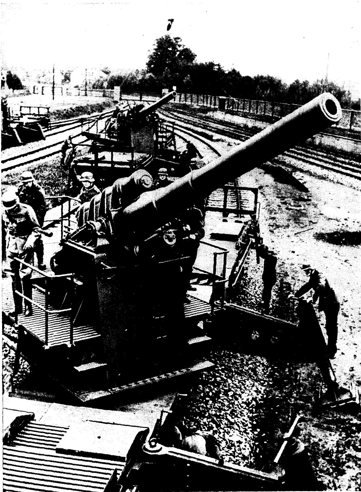
Figure 76.—150-mm railway guns being emplaced.
