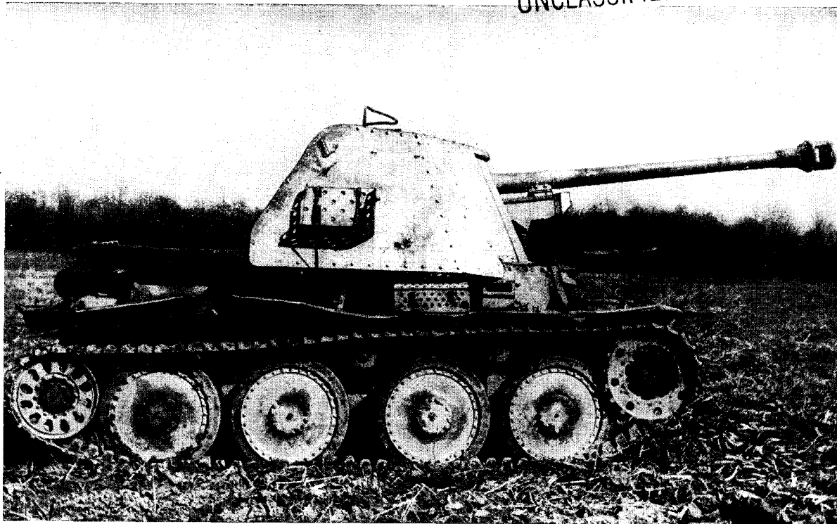
Figure 82.—7.5 cm Pak 40 on Pz. Kpfw. 38 (t) Chassis.
