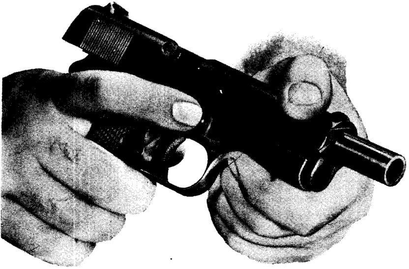
Figure 26. Removing slide stop pin from pistol M1911A1.
