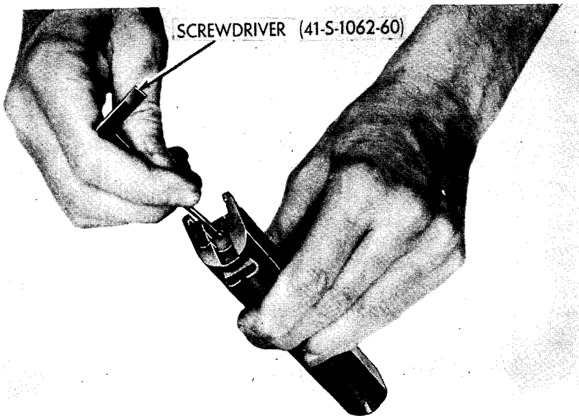
Figure 28. Removing firing pin stop.
