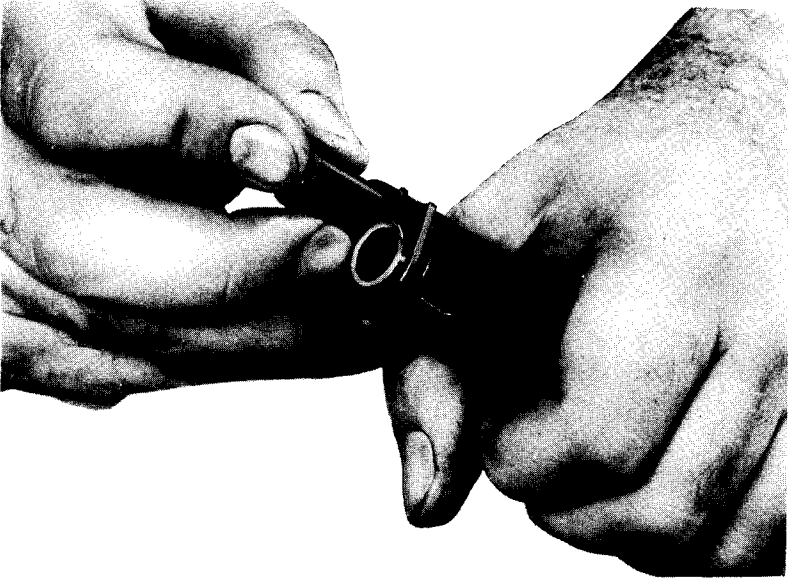
Figure 24. Removing recoil spring plug from pistol M1911A1.
