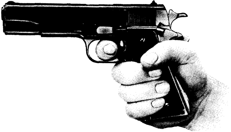
Figure 10. Pistol M1911A1, hammer at half cock position notch, finger squeezing trigger.
