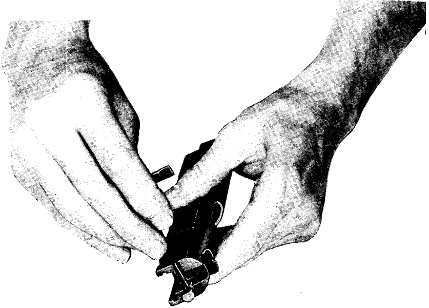
Figure 30. Removing extractor from slide.
