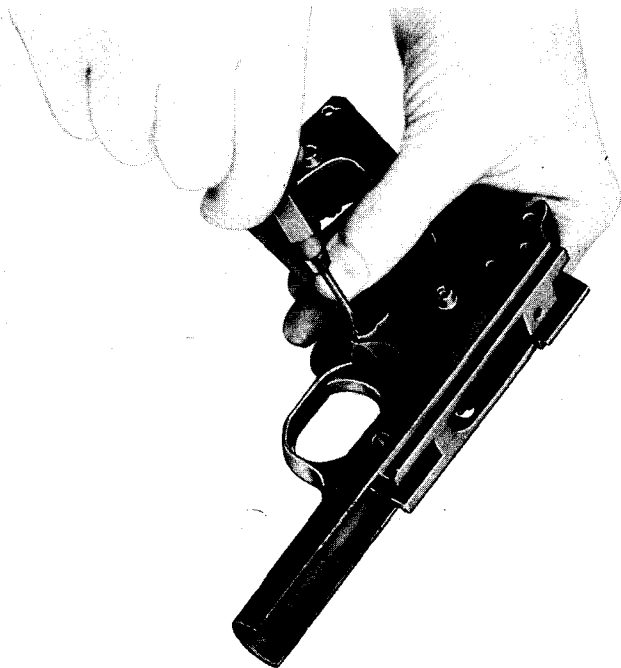
Figure 45. Disassembling new design magazine catch from receiver
