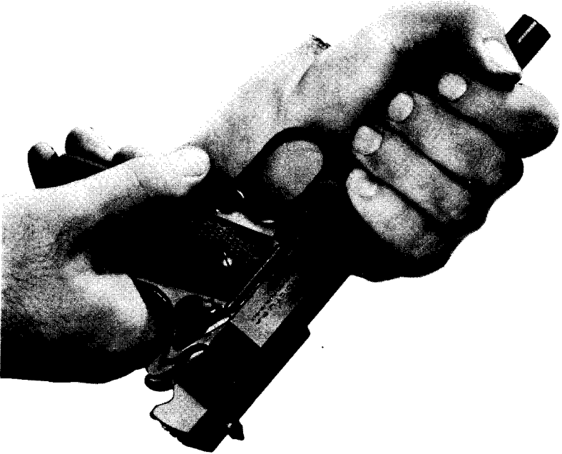
Figure 25. Lining up slide stop of pistol M1911A1.
