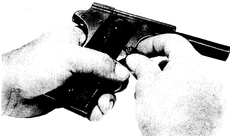
Figure 46. Disassembling old design magazine catch from receiver.
