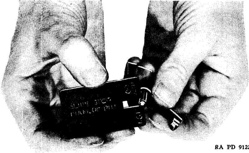
Figure 39. Checking slide stop pin.
