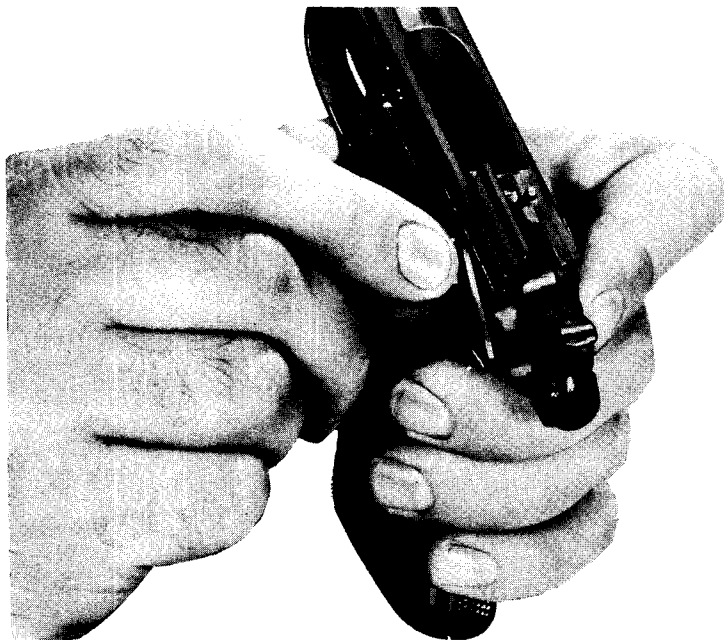
Figure 43. Removing safety lock.
