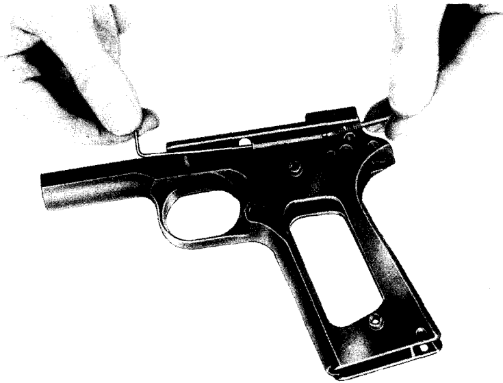
Figure 47. Removing slide stop and safety lock plunger assembly.
