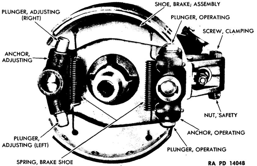
**Figure 61 – Top View of Brake Mechanism Assembly**
