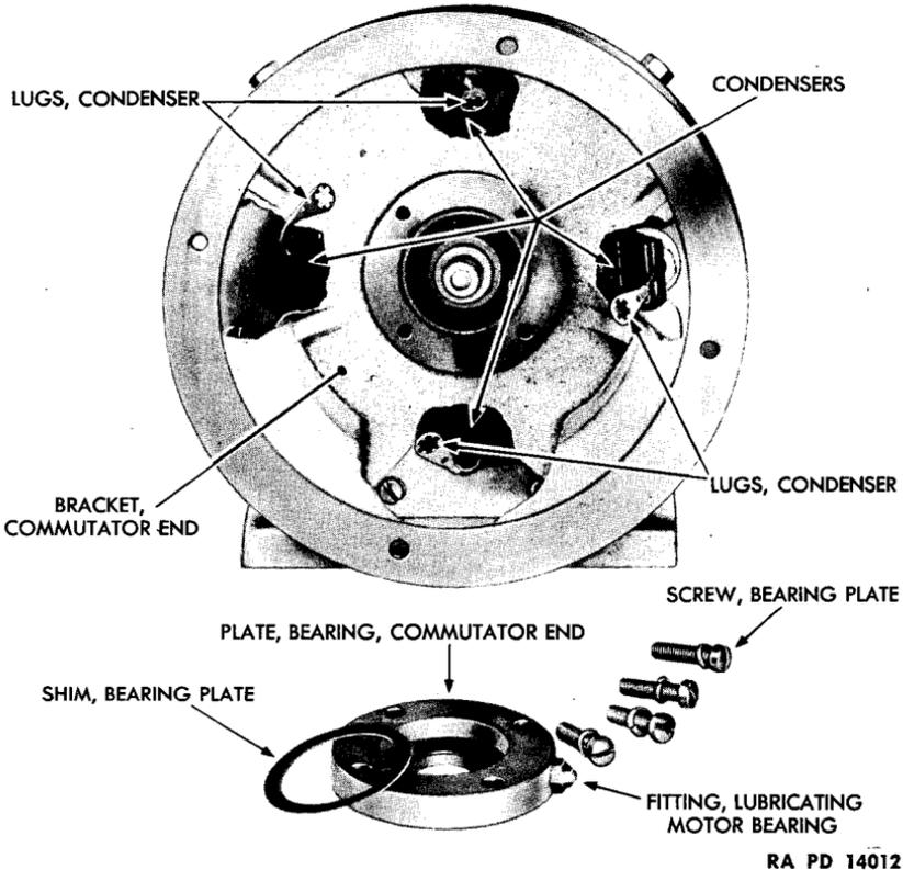
**Figure 15 — Commutator End Bracket With Bearing Plate Removed**
