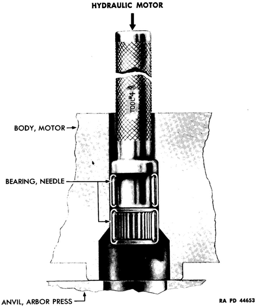
Figure 48 – Removal Of Shaft Needle Bearing From Motor Body
