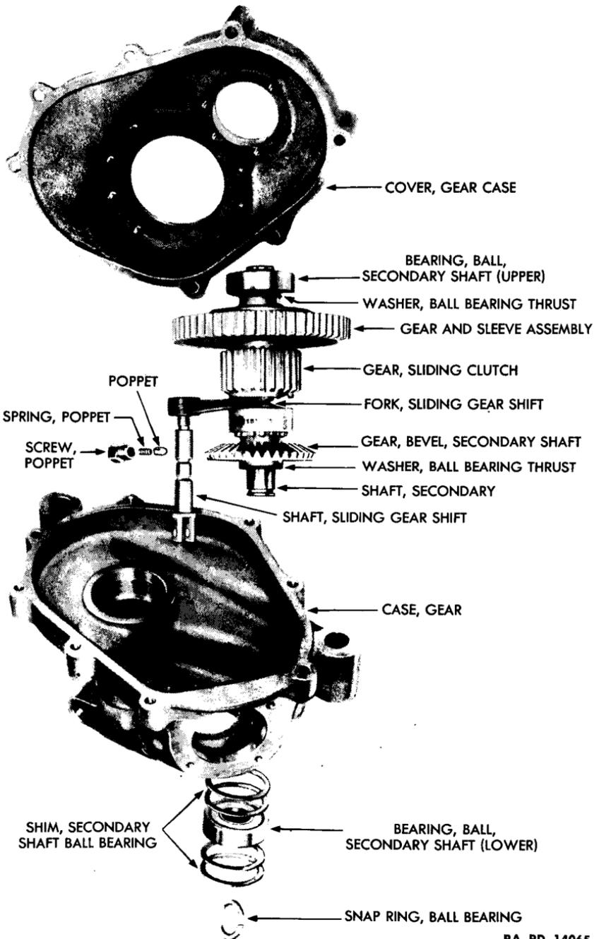
Figure 77 — Gear Case With Secondary Shaft Partly Assembled
