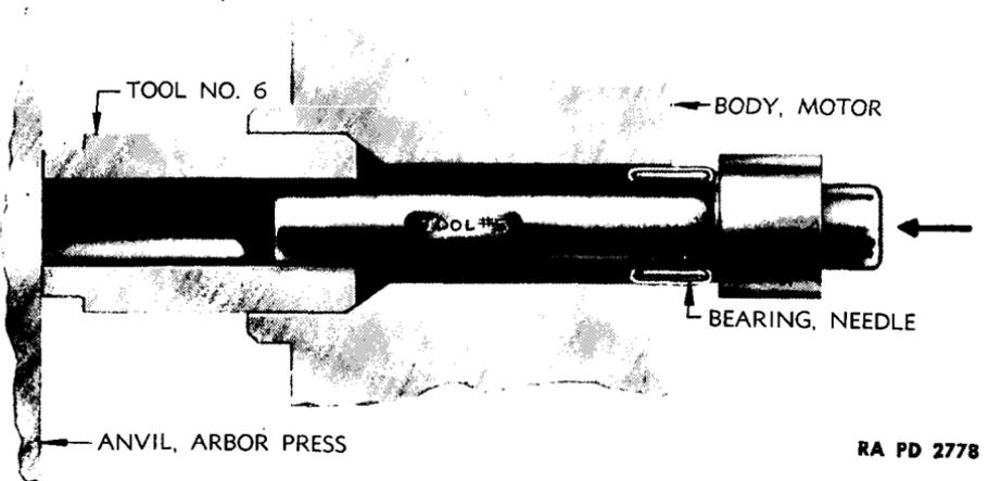
**Figure 51 – Installing Shaft Inner Needle Bearing In Motor Body**
