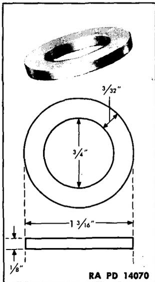
Figure 83 – Special Tool Washer
