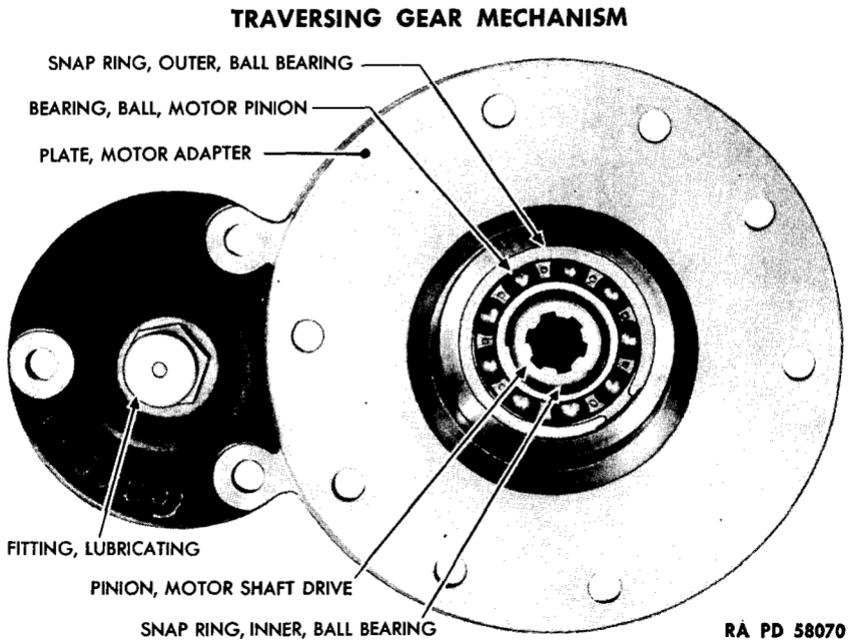
**Figure 69 – Motor Adapter Plate Assembly – Top View**
