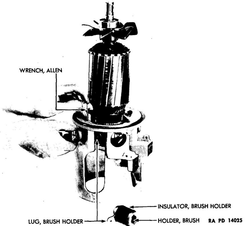
**Figure 28 – Installing Brush Holders**
