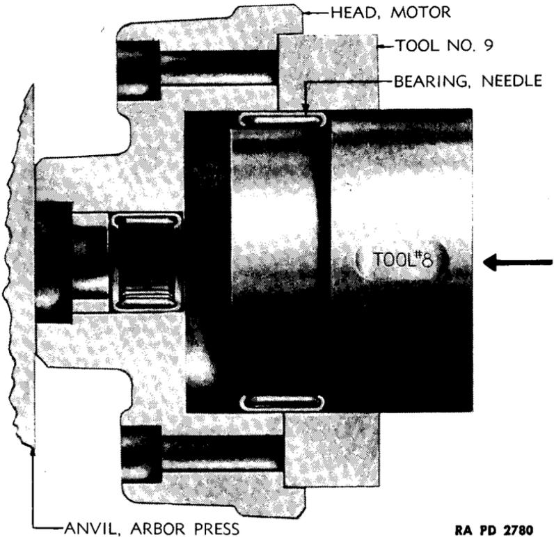
**Figure 53 – Installing Gerotor Needle Bearing In Motor Head**
