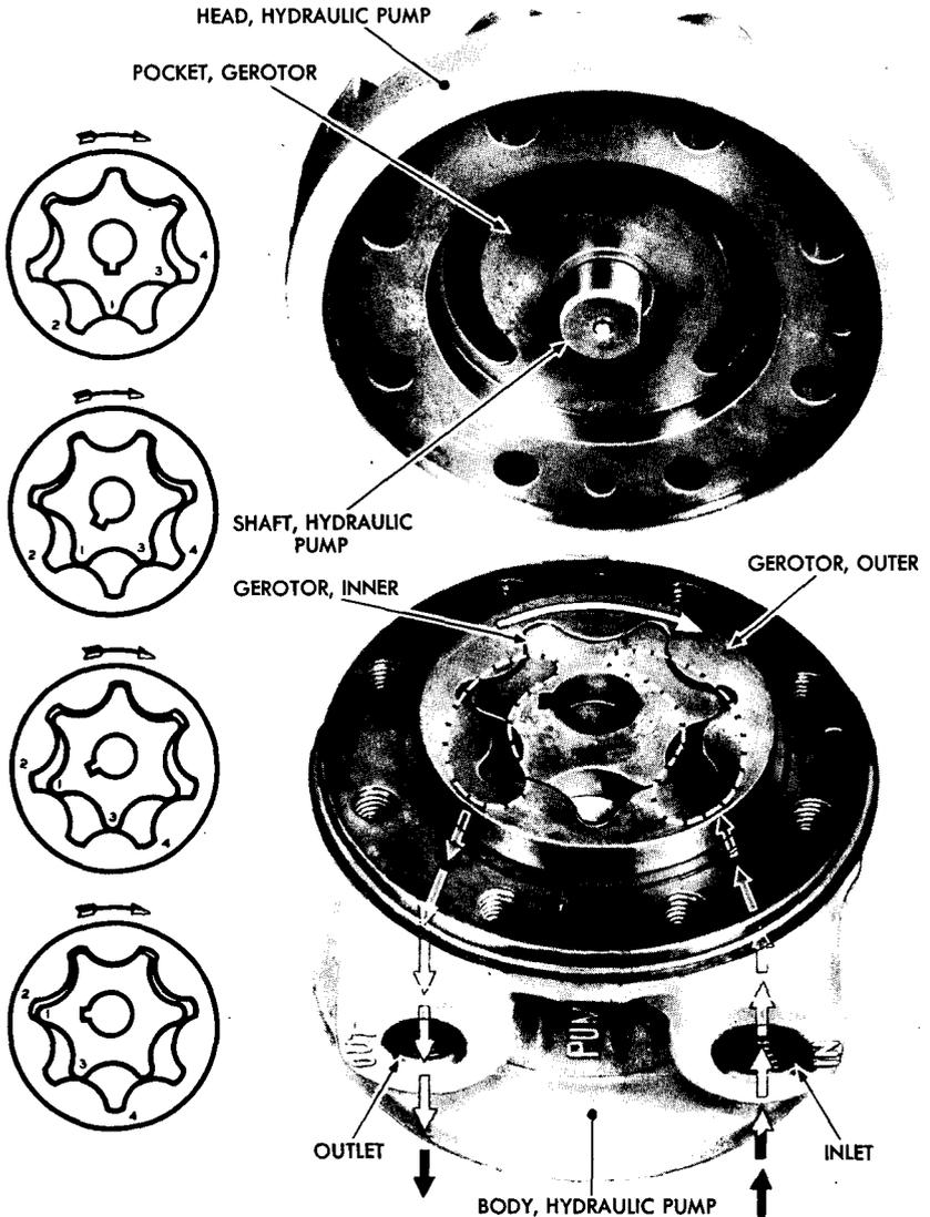
DIAGRAM OF HYDRAULIC PUMP, PARTLY DISASSEMBLED. LONG ARROW SHOWS DIRECTION IN WHICH GEROTORS ARE ROTATED BY SHAFT. SHORT ARROWS SHOW HOW OIL IS DRAWN THROUGH SUCTION PORTS AND SQUEEZED OUT THROUGH PRESSURE PORTS. SMALL DRAWINGS SHOW HOW ROTATION OF INNER GEROTOR IS TRANSMITTED TO OUTER GEROTOR.
