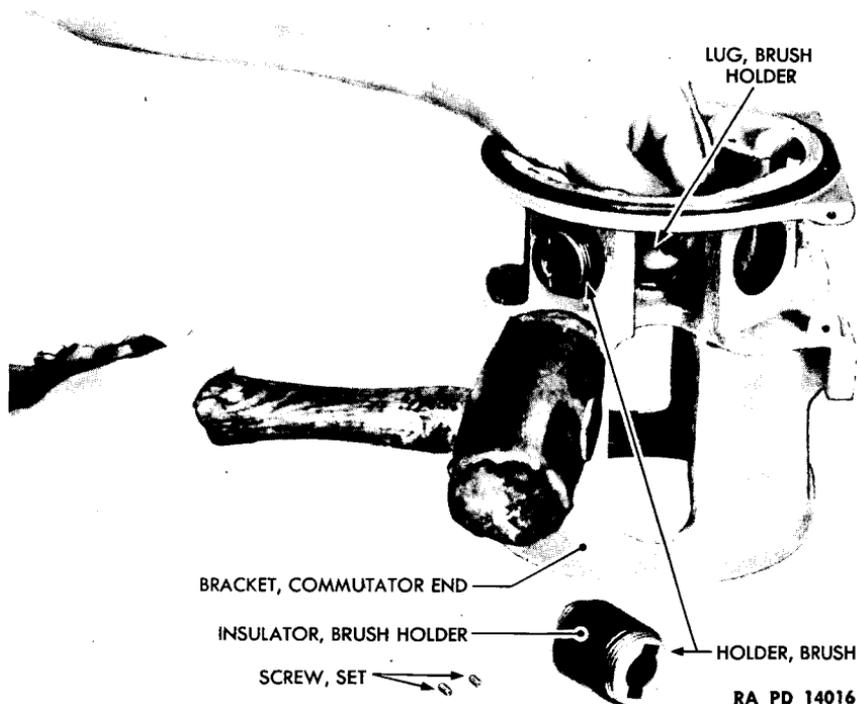
**Figure 20 — Removing Brush Holders From Commutator End Bracket**
