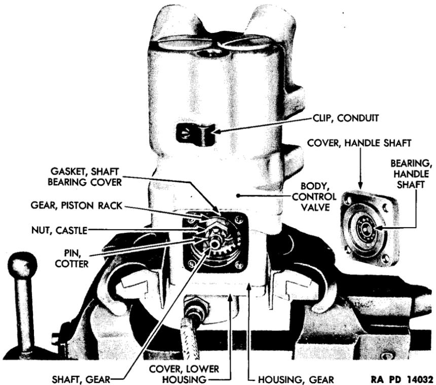
**Figure 36 – Valve Body And Gear Housing
