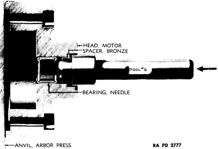
**Figure 50 – Installing Bronze Spacer In Motor Head**
