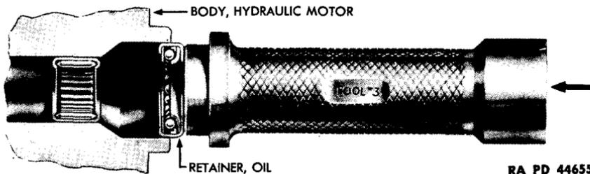
*Figure 54 — Installing Oil Retainer In Hydraulic Motor Body*
