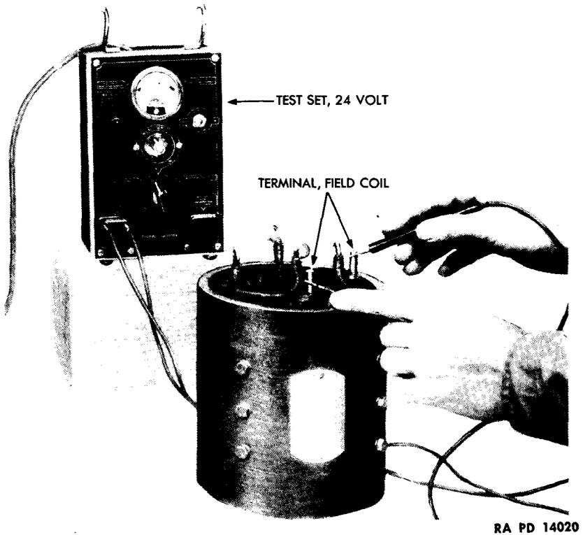
**Figure 25 — Checking Field Coils For Open Circuit**
