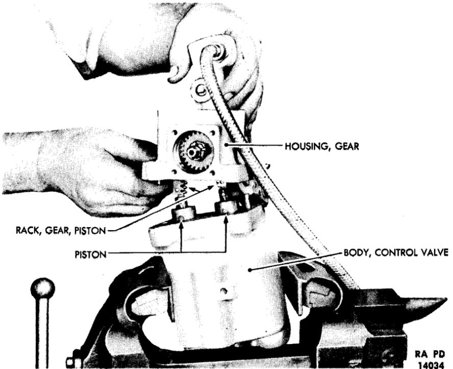
**Figure 38 — Removing Gear Housing, Handle, And Piston Assembly From Valve Body**
