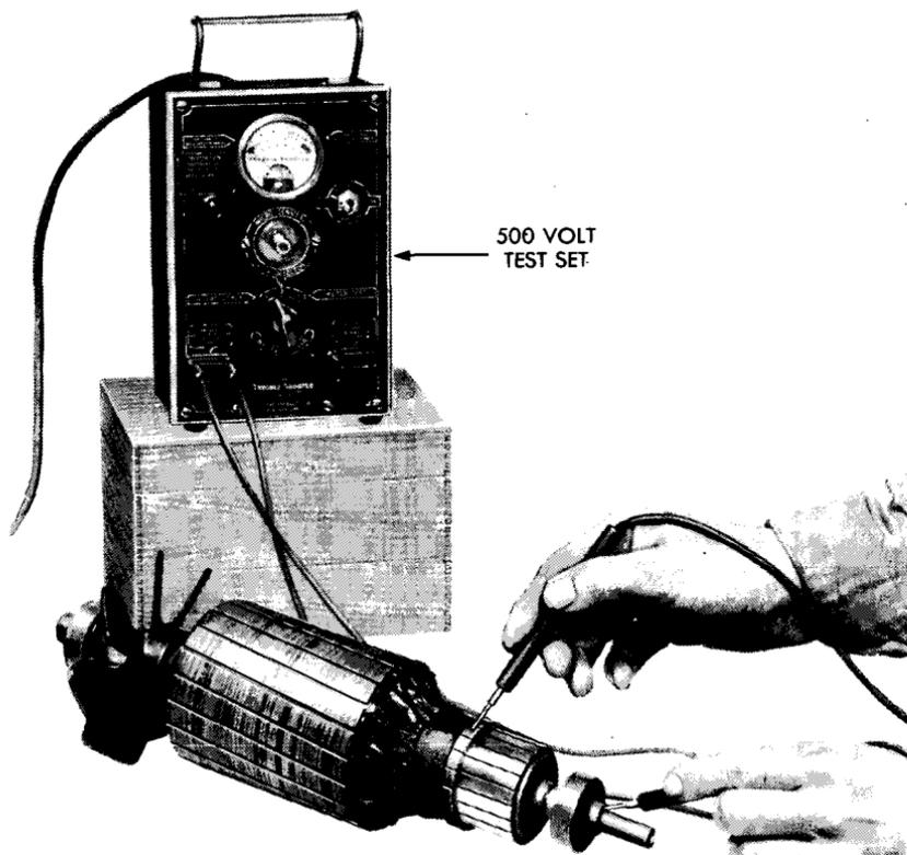
**Figure 22 — Testing For Ground In Armature** RA PD 14017
