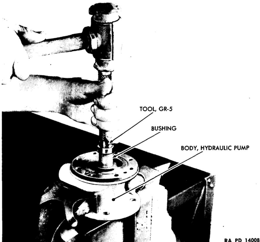
**Figure 10 — Assembling New Bushing In Pump Body**
